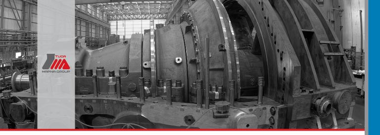
In special cases, an inspector can even enter the turbine via the opening on the exhaust casing through which the condenser-side bearing is normally mounted and dismounted. In this case, the inspection can take place without removing the casings. This enables the inspector to check closely for any probable damage to the last stage rotary blades.
