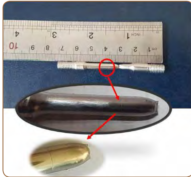
Figure 6- Brazed sample after tensile test
