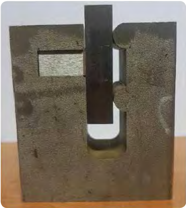
Figure 13- Bulk shear test sample after brazing
