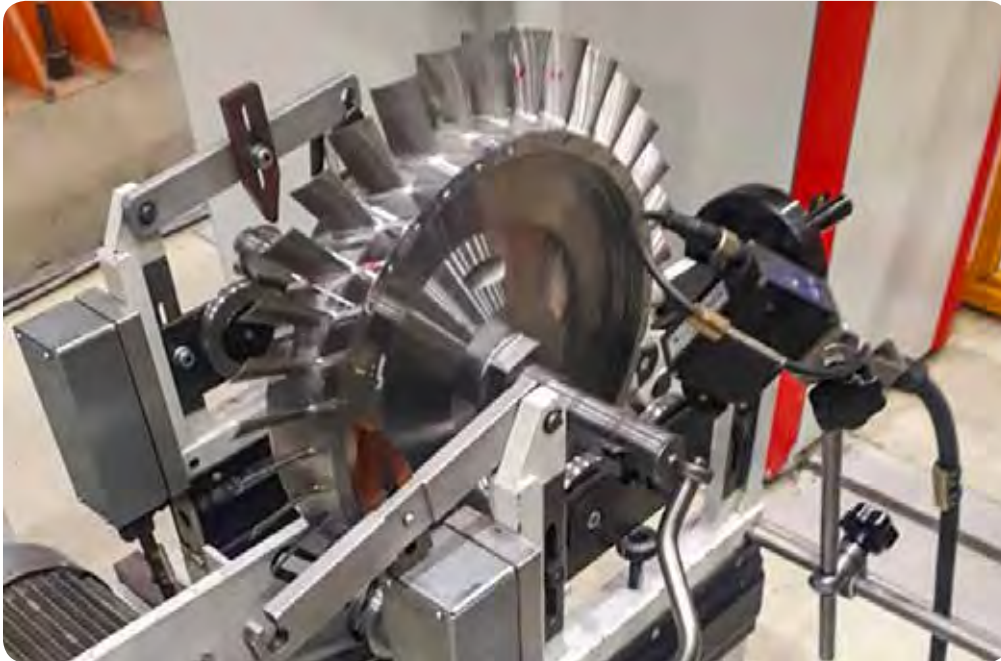
Figure 7- Bladed disc balance procedure
