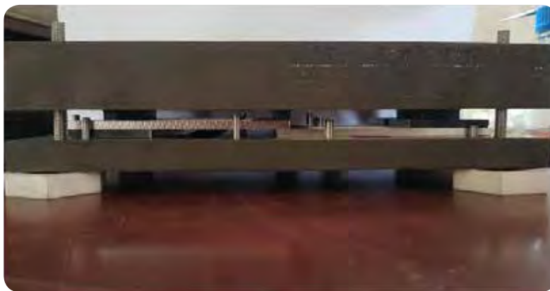
Figure 11- Shear test sample in brazing fixture
