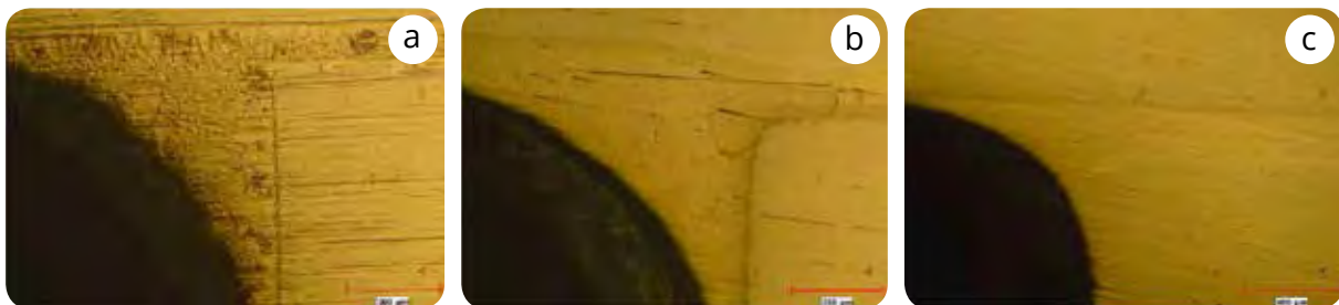
Figure 4- a) Ni based filler (BNi-2) b) Au based filler (BVAu-4) c) Pa based filler (PGK-1000)
