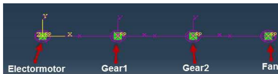
Fig. 4 – Entire ACC gearbox system mass-spring model
