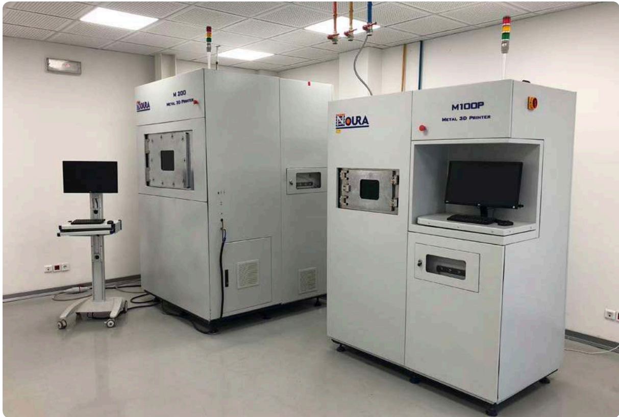
Fig. 4 – Installed SLM machines at MAPNA Turbine additive manufacturing laboratory
