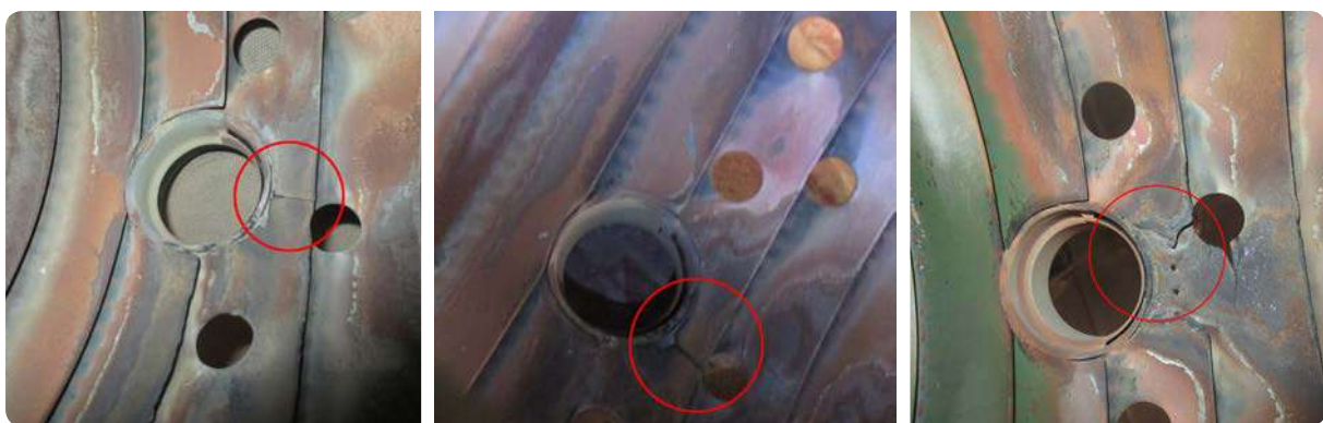
Fig. 2 – Damages occurred in the combustor liner of the industrial gas turbine
