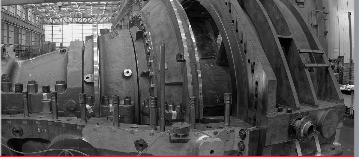
In special cases, an inspector can even enter the turbine via the opening on the exhaust casing through which the condenser-side bearing is normally mounted and dismantled. In this case, the inspection can take place without removing the casings. This enables the inspector to check closely for any probable damage to the last stage rotary blades.
