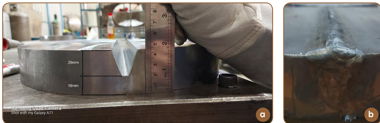
Figure 4 - (a) Dimensional specifications of test plates, (b) One typical completed test plate
