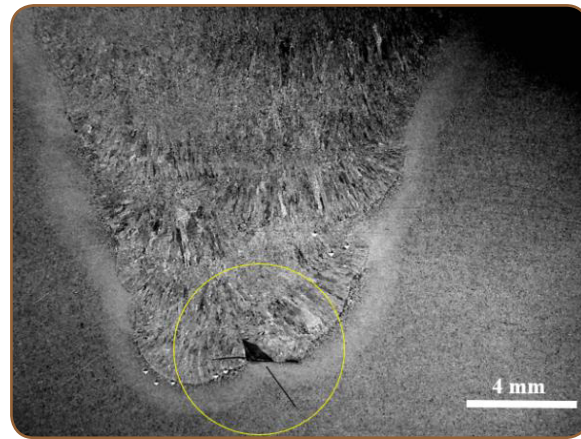
Figure 7 - Macrographic image of the PWHT sample. The marked area indicates the location of a defect in the root
