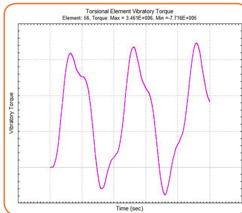
Figure 6 - Faulty torque in the shaft journal
