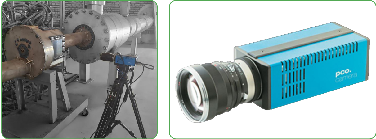
Figure 6 - Imaging system comprising a high-speed camera and an optical lens
