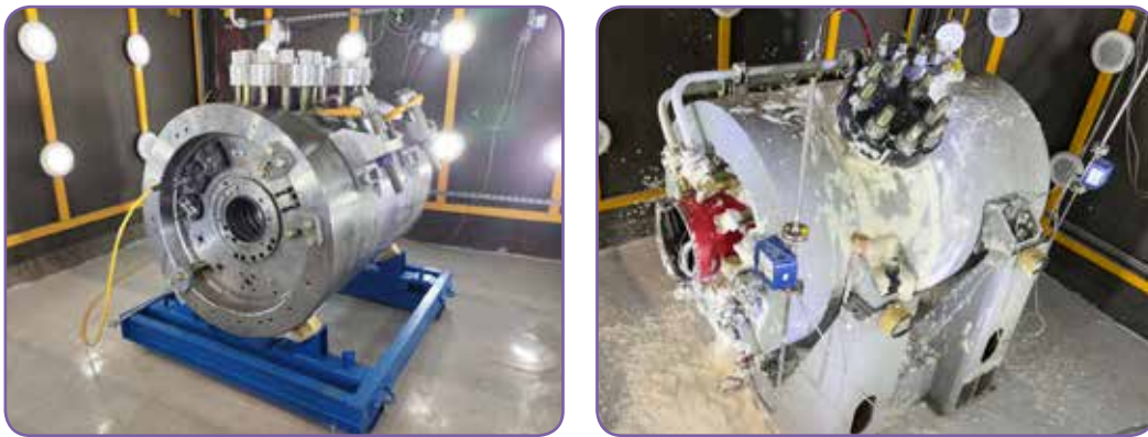
Figure 5- Gas Leakage Test of LP and HP Compressors
