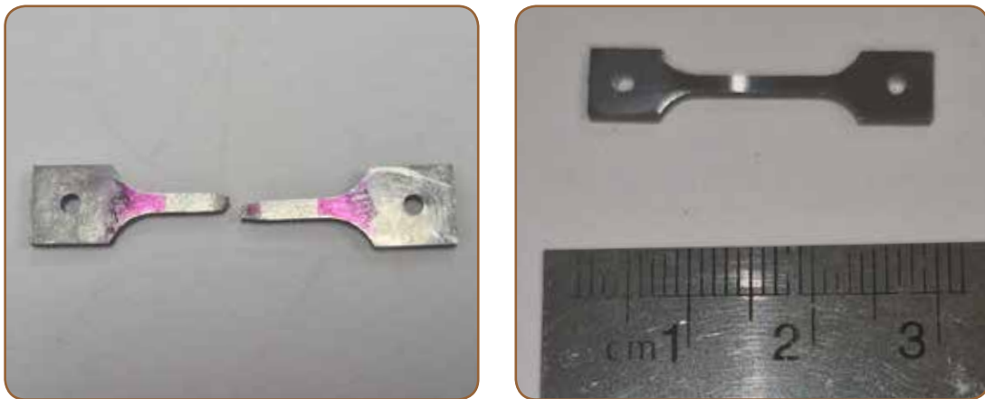
Figure 6- Pin-Loaded Specimen before and after Testing
