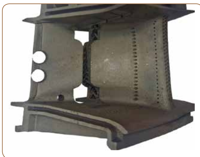
Figure 10- Extraction of Small Specimens from a Turbine Blade
