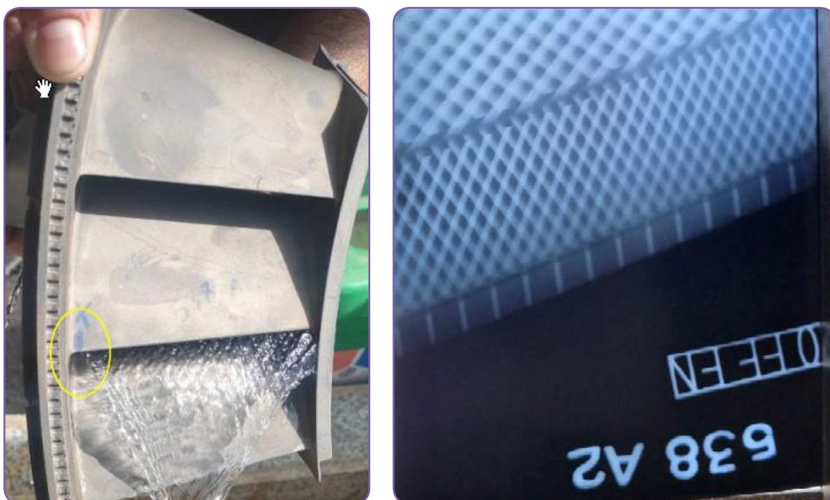
Figure 10 - Examination of the cooling flow path for 2 nd stage nozzle vane using water flow test and radiographic testing (RT)
