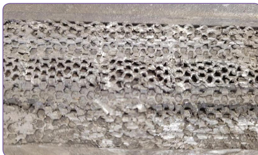
Figure 3 - Honeycomb seal area on a 2 nd stage nozzle vane of MGT-30 after first overhaul duration
