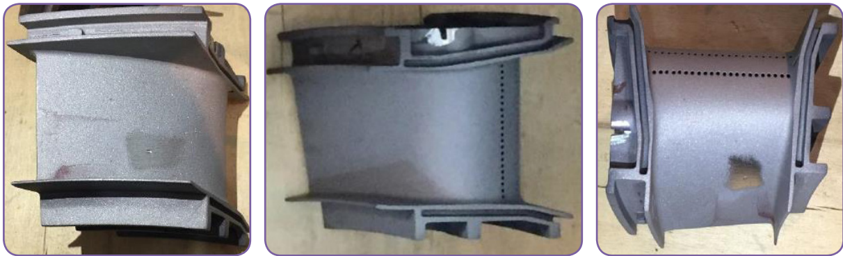
Figure 4 - A 1 st stage nozzle vane of MGT-30 after defect removal by grinding
